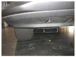
6. Attach the 3.75 x 3.5 sleeve and lower scoop using the #60 clamps
