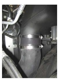
5. Attach the remaining #64 clamp onto the upper half of the scoop.
