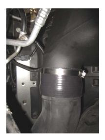
1. Attach the 4 x 3 sleeve to the volant box and tighten the #64 clamp.
