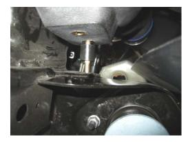
3. Align the rubber bumper with the existing hole on the frame.
