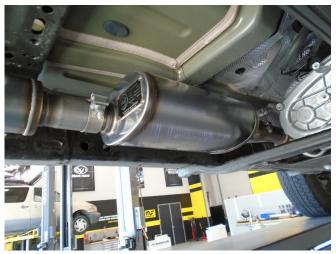
Begin installation of your new MAGNAFLOW system by attaching the Muffler Assembly to the catalytic converter outlet using the OEM clamp. Engage the welded hanger to the rubbe insulators. Keep all fasteners and clamps loose until final adjustment.
