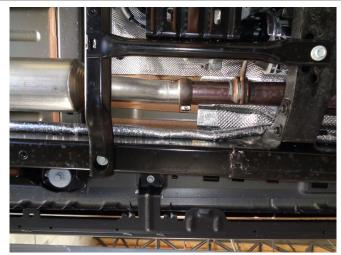
Begin removal of the OEM exhaust system by loosening the clamp attaching the exhaust to the catalytic converter.
