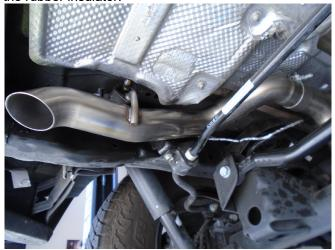
oosely install the Tailpipe Assembly to the Over-Axle Assembly using the supplied clamp. Locate the welded hanger to the rubber insulator.
