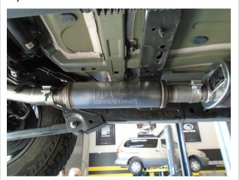
Next attach the Resonator Assembly inlet to the Muffler Assembly outlet using the supplied clamp.
