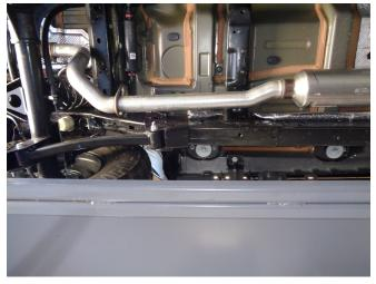
With the system supported, working front to rear disengage the hangers from rubber insulators and remove the OEM system. Do not discard or damage the clamp or rubber insulators as they will be used to install the new system.
