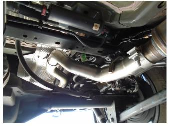
Next loosely install the Over-Axle Assembly using the supplied clamp. Locate the welded hanger to the rubber insulator.
