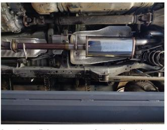
**Step 3:** Install the new system by attaching inlet pipe and muffler assembly with the supplied hardware.
