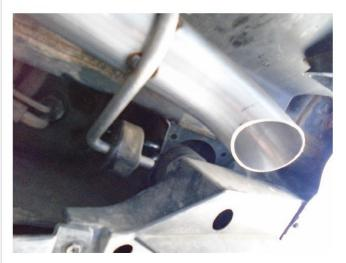
**Step 6:** Using the OE rubber insulators install the tailpipe assemblies to the Over Axle Pipe fitting the hangers into the installed hanger brackets.
