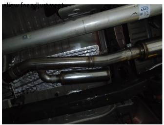
Step 4. Install the Outlet Resonator Assembly by attaching the inlet pipe to the outlet of the Inlet Resonator Assembly. Loosely secure using the supplied band clamp.
