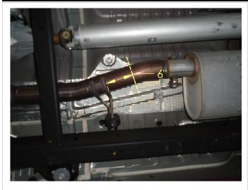
Step 1. The muffler section will need to be removed from the OEM exhaust system. Using a Sawzall or similar cutting tool cut the exhaust pipe 6" rearward of the welded hanger in front of the muffler.
