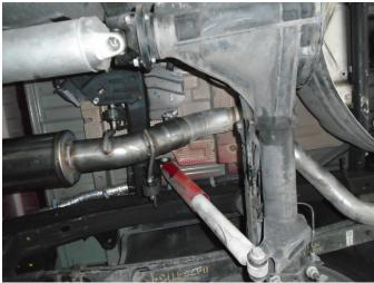
Step 5. Slip the Outlet Resonator exit pipe over the cut OEM rear pipe. Loosely secure using the supplied band clamp. Engage the welded hangers to the rubber
