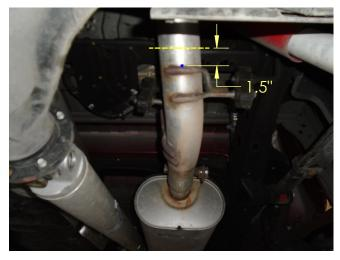
Step 2. Next cut the exhaust rearward of the muffler 1.5" behind the welded hanger. Disengage the welded hanger on the muffler from the rubber insulators. Remove the muffler section. Deburr the sharp edges from the cut ends. You are now ready to install your new MAGNAFLOW system.
