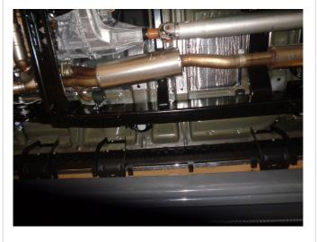
Step 2: Next loosen the clamp rearward of the OEM resonator. Detach all welded hangers from the rubber insulators. The system may now be removed. Be sure to retain all mounting hardware as it will be needed to install your new MAGNAFLOW system
