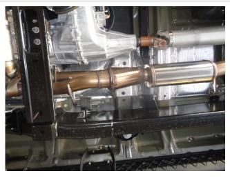
Step 4: Begin installing your new system by loosely attaching the Muffler Assembly to the catalytic converter outlet pipes using the OEM hardware. Engage the welded hanger to the rubber insulator.
