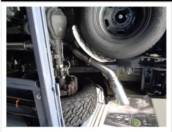
Step 6: Finish by loosely attaching the Tail Pipe Assembly using the supplied clamp. Install the welded hanger to the rubber insulator.
