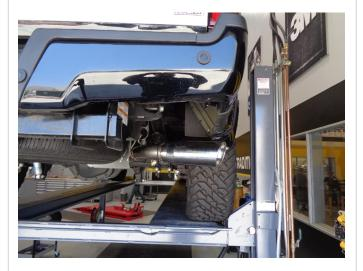
Step 7: Once a final position has been chosen for the new exhaust system, evenly tingten all clamps from front to rear using the torque specifications on page one of these instructions. Inspect all fasteners after 25-50 miles for operation and re-tighten if necessary.
