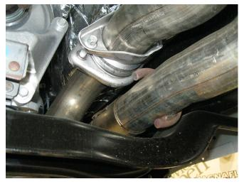
Step 1: To remove the OEM system loosen the clamp at the inlet pipe junction to the catalytic converters. Next, unbolt the flange coupling at the other inlet pipe.
