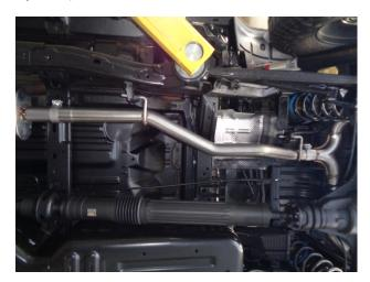
Step 3. Install this to the Inlet Pipe Assembly using the supplied 3.00" clamp and attaching the hangers, then attach the Y-Pipe Assembly to the Extension Pipe.
