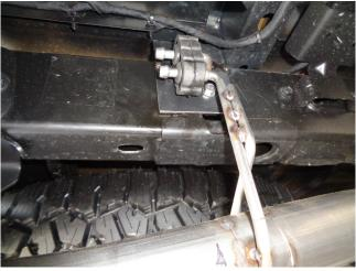
Step 5. As this vehicle was not setup for dual exhaust from the factory, a hanger bracket will need to be installed to the frame on the Passenger side with the supplied hardware as shown. Use the supplied zip tie to move the breather tube out of the way.
