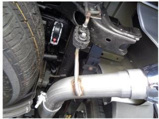
**Step 5.** from the factory, hanger brackets will need to be installed. Install the hanger brackets on the rear frame section using the supplied fastener hardware as shown
