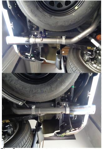
Step 6. Using the supplied rubber insulators install the Tailpipe Assemblies to the Extension pipes fitting the hangers into the installed hanger brackets.
