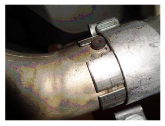
Step 2: To install the MagnaFlow Muffler Assembly slide the inlet onto the OE outlet making sure to align the slot with the peg on the outlet pipe. Secure with the supplied 3.00" clamp.
