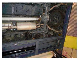
Step 1. Begin removal of the OE muffler by loosening the three clamps attaching the exhaust to OE system. Disengage the hangers from the rubber insulators and remove the muffler. Do not discard or damage the rubber insulators as they will be used to install the new system.
