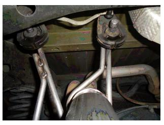
Step 3: insert the welded hangers into the rubber insulators
