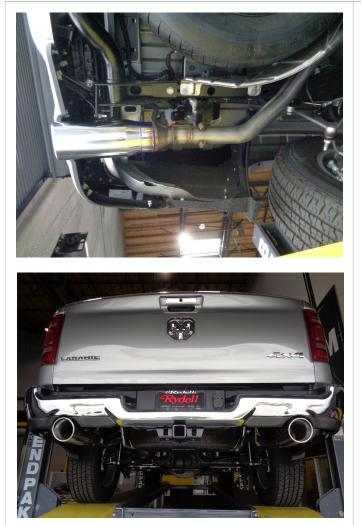
Step 5: Once a final position has been chosen for the new exhaust system, evenly tighten all clamps from front to rear using the torque specifications on page one of the instructions. Inspect all fasteners after 25-50 miles of operation and re-tighten if necessary.
