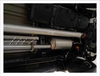
Step 1: To remove the OEM exhaust system, loosen hardware at the muffler flange.
