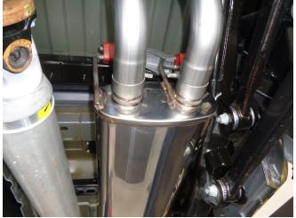
Step 4: Locate the welded hangers to the rubber insulators. Leave all clamps loose for final adjustment of the complete syste once installed.
