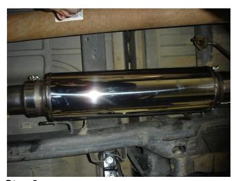
**Step 3.** Loosely attach the Muffler Assembly using the supplied clamps.
