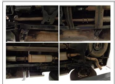
**Step 1.** Working front to rear loosen or remove all OEM band clamps and disengage all welded hangers from the rubber insulators. Be sure to retain all mounting hardware as it will be needed to install your new MAGNAFLOW system.
