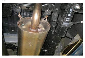
**Step 2.** Disengage hangers from rubber insulators and remove the OEM exhaust.
