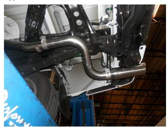
**Step 4.** Attach the Tail Pipes to the system using the supplied 2.50" clamps. Install the tips using a similar fashion.
