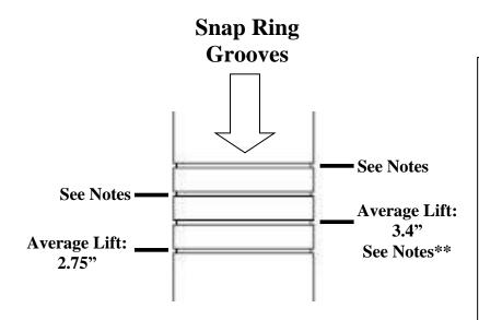
**Important:** Ensure that the snap ring is fully seated in the snap ring groove (you should be able to rotate the snap ring manually/by hand). **Note: Improper installation will cause permanent damage to the shock. Please refer to the Pro Truck Sport Damper instructions for more info regarding proper installation and fitment.**
