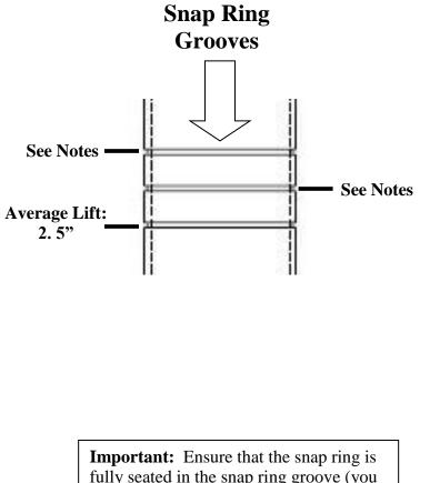
fully seated in the snap ring groove (you should be able to rotate the snap ring manually/by hand). Note: Improper installation will cause permanent damage to the shock. Please refer to the Pro Truck Sport Damper instructions for more info regarding proper installation and fitment.
