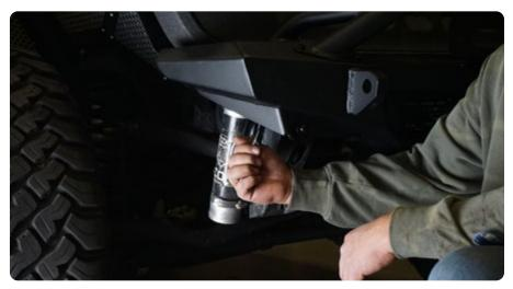
**STEP 12** | If you are running a winch and fairlead, install it at this time using the hardware provided with the winch and fairlead.
