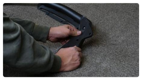
STEP 7 | Loosely install bull bar onto the bumper using the provided M8x25 allen head hardware.
