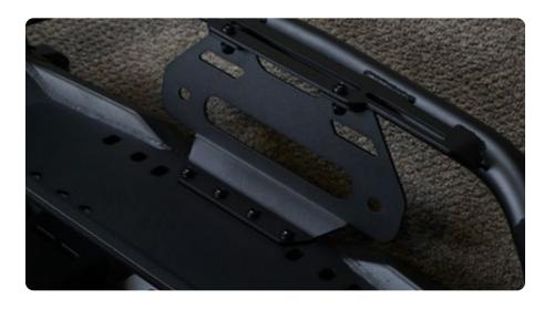
**STEP 9** Install flat nuts on the bumper by sliding them into place. These can sometimes require a little force to install.
