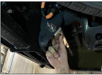
**6.** Align and slide the Hanger Plate over the Bolts. Then start threading the Nuts onto the Bolts.
