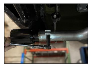
22. Locate 1 of the CORSA Tip Assemblies and 1 – 2.75in Clamp from the Hardware Kit. Slide the clamp over the outlet of the Tail Pipe
