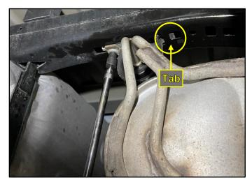
3. Locate the Middle Factory Grommets and use a 10mm Socket & Ratchet with an Extension or Wrench to remove the Bolt that attaches it to the Frame. Pull the Factory Grommet toward where the Bolt was attached. This releases a tab from a hole in the Frame.
