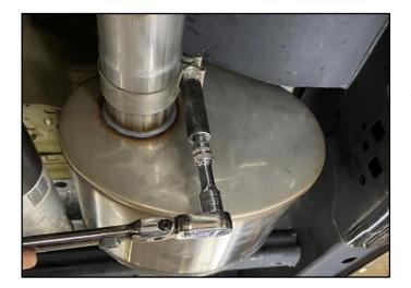
17. Use a 15mm Socket & Ratchet or Wrench to SNUG the Clamps connecting the CORSA Muffler to the Mid Pipe and the Mid Pipe to the Tail Pipe.
