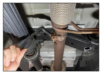
Use a 15mm Socket & Ratchet or Wrench to loosen the Stock Clamp, connecting the Front Section and Rear Section of the Stock exhaust.
