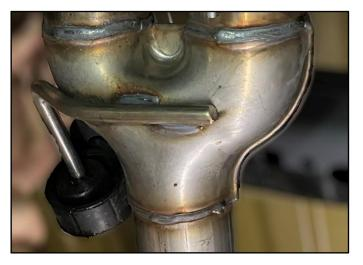
Install the Factory Grommet from the rear of the Factory to the Hanger on the Wye of the CORSA Mid Pipe
