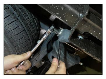
Using a 13mm Socket & Ratchet and Wrench or 2 - 13mm Wrenches, SNUG the Rear Hanger Bolts and Nuts.
