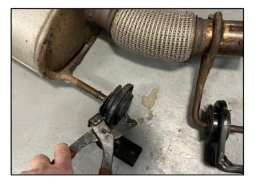
1. Using Grommet Pulling Pliers or similar, remove the 2 Factory Grommets from the Factory Muffler and 1 from Head Pipe (if equipped with Flex).
