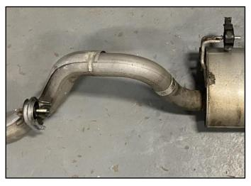
**3.** Remove the Factory Grommet(s) using Grommet Pulling Pliers or similar from the rear of the Factory Muffler and Tail Pipe.
