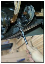
2. Use a 10mm Socket & Ratchet or Wrench to remove the 2 Bolts on each of the Factory Grommets. If the Factory Exhaust has a Flex Section, there are two Grommets. If the Factory Exhaust does not have a Flex Section, there is one Grommet and may look different than shown.
