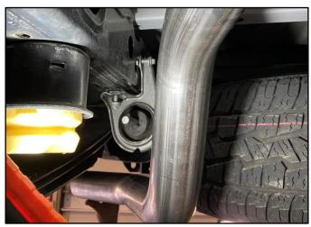
**14.** Locate the bolts for the Rear Factory Grommet from Removal Step 4 and 5. A second person may be needed to assist with this step.
