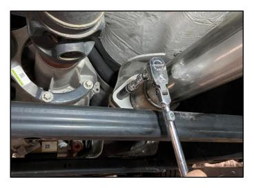
**6.** Locate the Head Flange Bolts from Removal Step 7. A second person may be needed to assist with this step.
