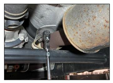
1. Use a 13mm Socket & Ratchet or Wrench to loosen the bolts from Stock Flange connection on the Front Section of the Stock exhaust. A second person may be needed to support the Front Section of the Stock exhaust.
