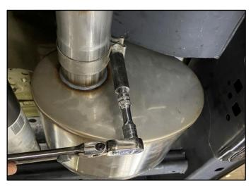
**15.** Use a 15mm Socket & Ratchet or Wrench to **SNUG** the Clamps connecting the CORSA Muffler to the Mid Pipe and the Mid Pipe to the Tail Pipe.
