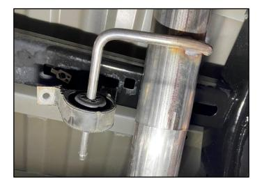
**13.** Locate the bolt for the Middle Factory Grommet from Removal Step 3. A second person may be needed to assist with this step.
