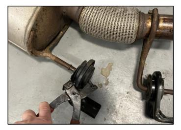
Remove the Factory Grommet(s) using Grommet Pulling Pliers or similar from the Factory Muffler and Head Pipe (if equipped with Flex).
