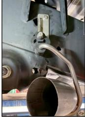
13. Locate the Isolator in the Hardware Kit. Insert the Isolator onto the CORSA Tail Pipe Hanger, then insert the other side of the Isolator on to the Frame Hanger.
