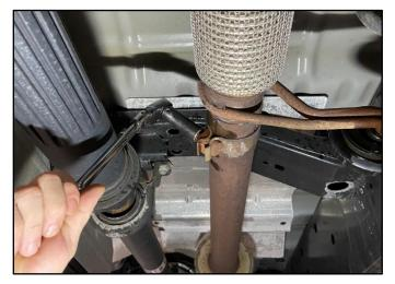
Use a 15mm Socket & Ratchet or Wrench to loosen the Stock Clamp, connecting the Front Section and Rear Section of the Stock exhaust.
