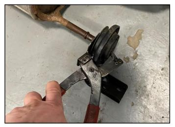
1. Using Grommet Pulling Pliers or similar, remove the Factory Grommets from the front of the Factory muffler. Note the orientation for the next step.
