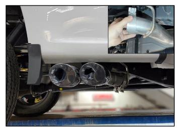
15. Locate 1 – 3in Clamp from the Hardware Kit. Install the Clamp as shown, with the Clamp Nut on top, facing away from the vehicle frame.
