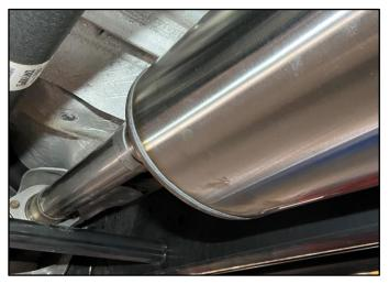
**9.** Locate 1 – 3in Clamp from the Hardware Kit and slide it over the Head Pipe. A second person may be needed to assist with this step.
