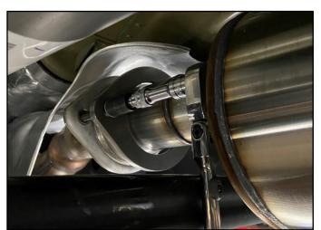
**10.** Locate the Head Flange Bolts from Removal Step 7. A second person may be needed to assist with this step.
