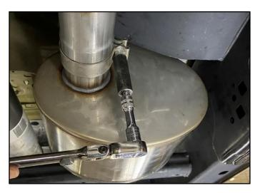
14. Use a 15mm Socket & Ratchet or Wrench to SNUG the Clamp connecting the CORSA Muffler and Tail Pipe.
