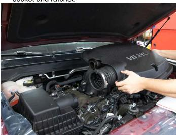
Carefully lift the engine cover along with the factory airduct and place it aside.
