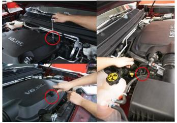
Use a 10mm socket and ratchet with extension to remove the three bolts shown above.
