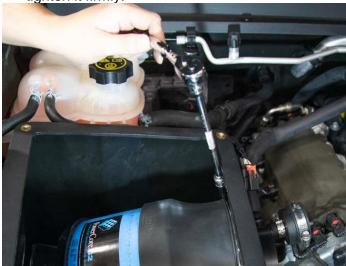
Insert the filter into the airbox and place it over the filter adapter. Tighten the filter clamp securely using an 8mm socket and ratchet.
