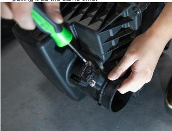
**11.** Remove the 2 Torx screws holding the factory MAF sensor using a T-20 Torx screwdriver.
