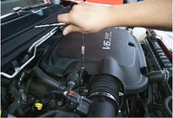
**3.** Loosen the clamp shown above using an 8mm socket and ratchet.
