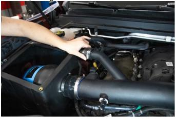
11. Insert the factory hose into the duct as shown.
