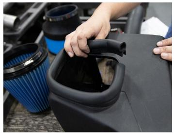
**3.** Insert the provided Bulb Seal to the Corsa airbox as shown.
