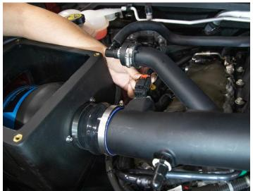
**13.** Insert the factory MAF sensor harness into the MAF sensor by pushing it firmly. Make sure to clip the red locking tab until a click is heard.
