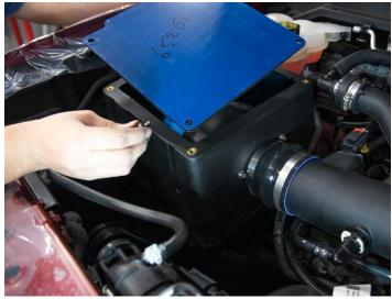
15. Remove the protective blue film and then place the Corsa lid over the airbox and secure it using the lid screws provided. Tighten the lid screws using a Philips head screwdriver. DO NOT overtighten.
