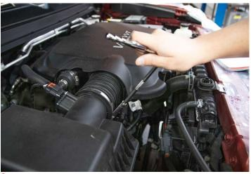
Loosen the duct clamp shown above using an 8mm socket and ratchet.
