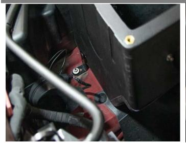
Use the provided bracket and secure it to the engine bay using the factory nut as shown above. Use a 10mm socket and ratchet to tighten it firmly.
