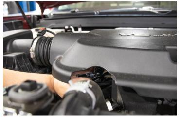
Unclip the vent line fitting by pressing on the side and pulling it gently.
