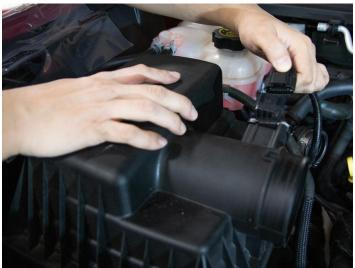
9. Unclip the factory MAF sensor harness by pulling on the tab till it clicks and then pressing it and pulling it as the same time.
