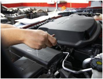
**5.** Loosen the throttle body clamp using an 8mm socket and ratchet.
