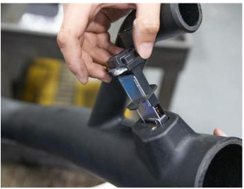
Insert the MAF sensor into the duct as shown with the MAF sensor gasket provided sandwiched between the MAF and the Duct.
