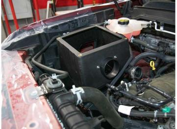
Carefully place the Corsa airbox as shown making sure to insert the fitting at the bottom of the airbox into the grommet in the engine bay.
