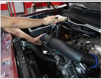
**14.** Tighten all the clamps using an 8mm socket and ratchet until the assembly is secure.
