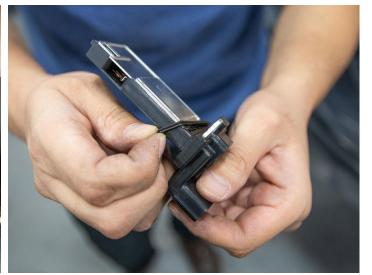
12. Remove the factory MAF sensor gasket shown above and place it aside. Keep the MAF sensor for use with the Corsa Air Intake.
