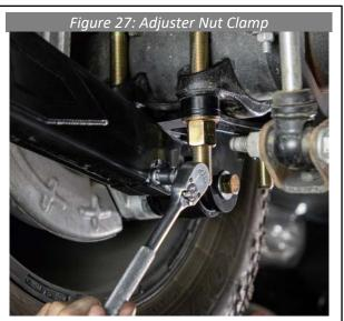
20. Do not exceed **2"** of thread showing from the face of the traction bar to the start of the threads on the eyelet (See Figure 28)
