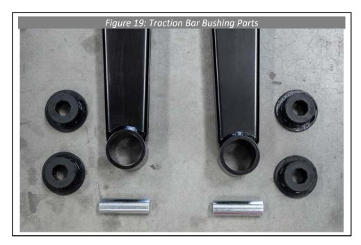
14. Install (2) traction bar bushings per traction bar from each side (Figure 20). A light lubricant, WD-40, may be used to install but do not grease the outside of the bushing. Once bushings are installed in traction bars, grease the inside bore of each bushing (Figure 21).
