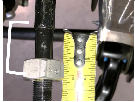
Figure 46b: Measure Position of Die
