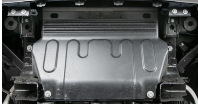
Figure 33: OEM Front Skidplate Reinstalled
