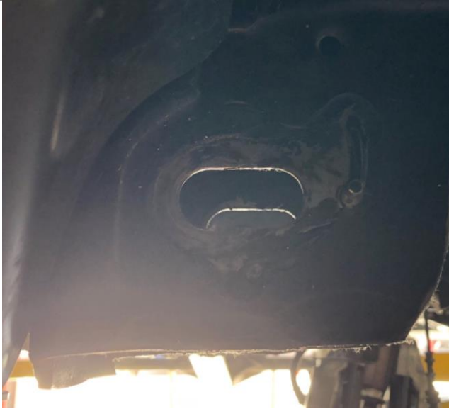
Figure 24g: Driver's Side Front Crossmember, After Trimming
