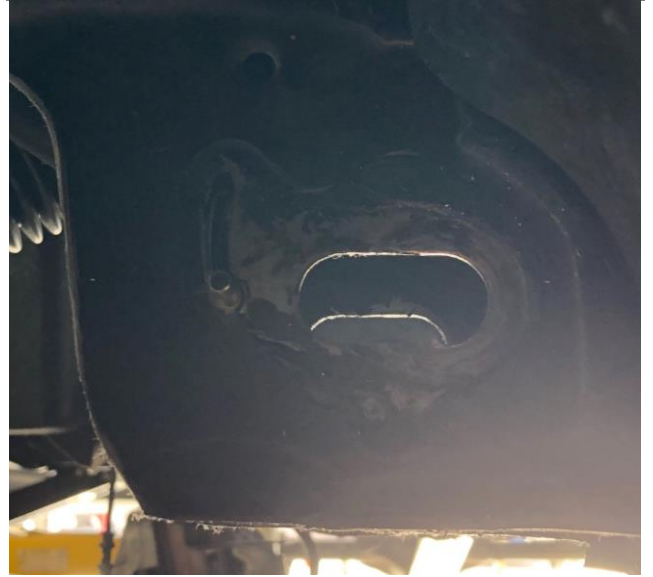
Figure 24h: Passenger's Side Rear Crossmember, After Trimming
