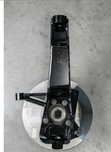
Figure 41d: Hub Installed in Cognito Spindle
