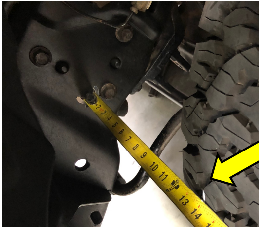
Figure 1: Measure from Frame Rail to Tire
