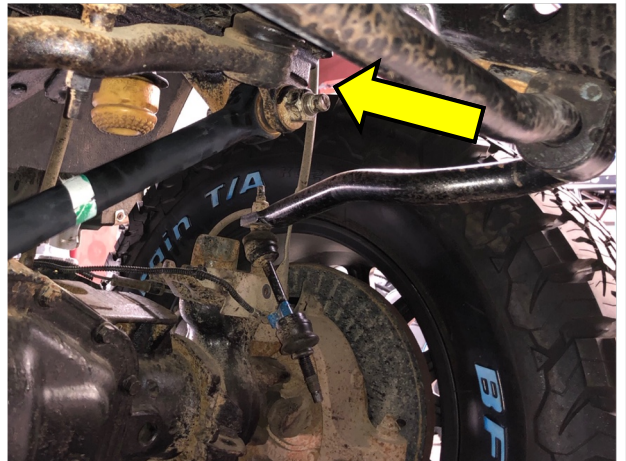
Figure 2: Remove Track Bar to Bracket Nut
