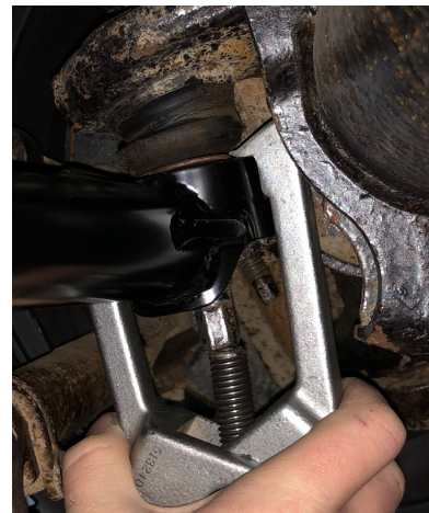
Figure 6: Remove Track Bar with Bearing Puller
