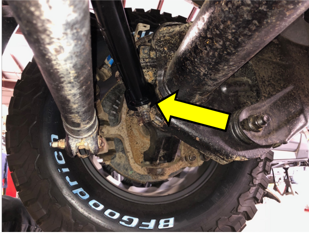
Figure 3: Track Bar to Axle Ball Joint Nut
