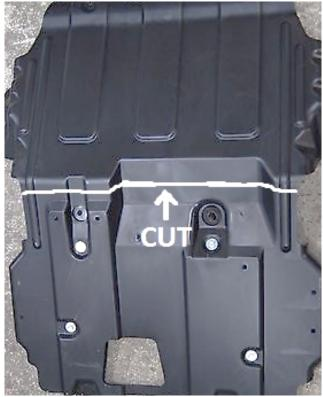
Figure 1: Make cut as shown, then trim to fit.
