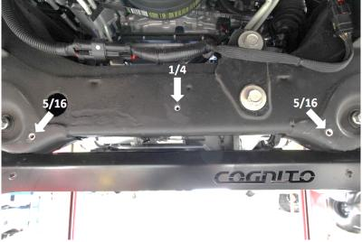
Figure 2: Insert 5/16 & 1/4 nutsert in the frame.
