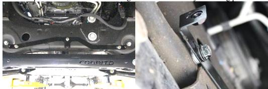
Figure 3: Bolt bracket to frame
