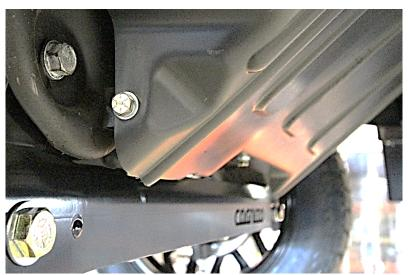
Figure 5: Drill out and bolt the skid plate to the mounting bracket
