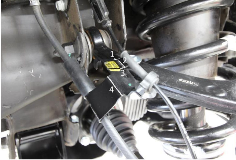
Figure 21: Brake line Mounting Bracket
