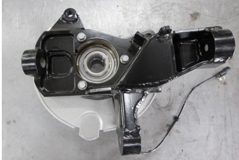
Figure 20: hub transferred to Cognito spindle
