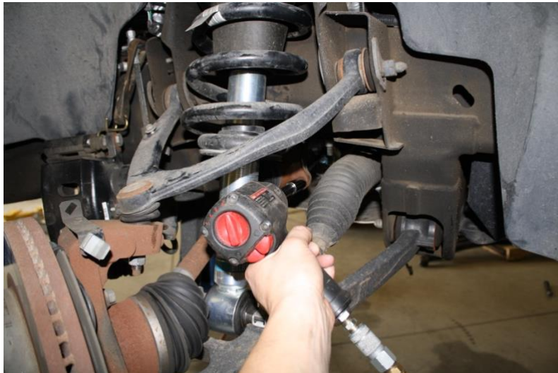
Figure 2: unbolt CV axle from differential
