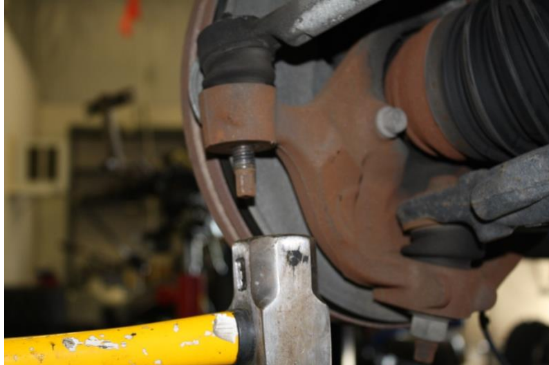
Figure 1: remove outer tie rod end from spindle
