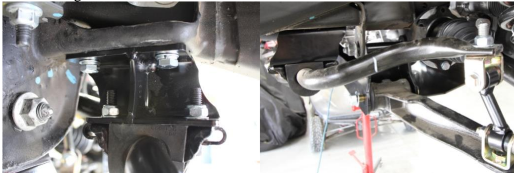
Figure 22: Sway Bar Spacer Bracket and Factory Sway Bar
