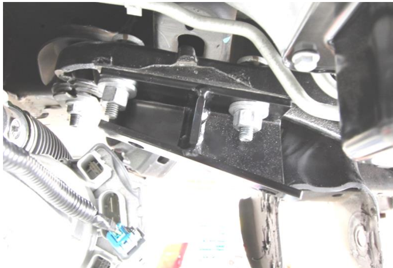
Figure 10: install passenger diff mount
