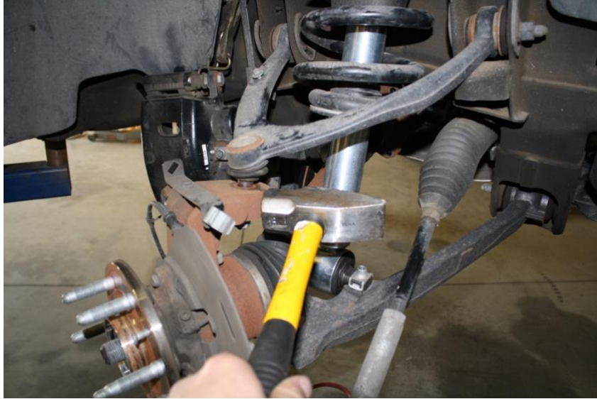
Figure 4: break loose upper ball joint, and lower ball joint
