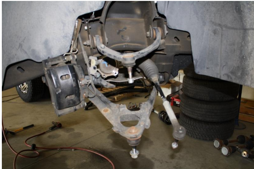
Figure 5: shock and spindle removed
