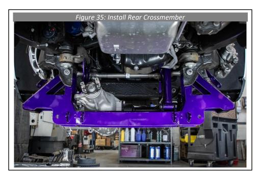
**47.** Skip this step for 2WD vehicle. Locate HP9123 and loosely fasten the passenger differential mount to the rear crossmember using the 1/2" x 3.5" Yellow Zinc Cap Screw (See Figure 36).
