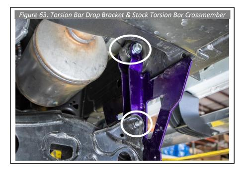
**92.** Using the holes on the Cognito torsion bar drop bracket flanges that sit on the bottom of the frame rail as a drill template, drill a 21/64" hole into the frame. Do this on both the passenger and driver side (see Figure 64).
