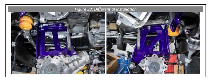
**44.** Skip this step for 2WD vehicle. To reconnect the rubber vent tube to the front differential, cut the bottom most tape holding the vent tube and differential wiring harness together. Open the hood and look near the fuse box, unclip the top of the vent tube from the harness it is attached to, and then go under the vehicle and pull down on the tube until it is long enough to be reconnected. Clip the top part of the vent tube back onto an appropriate harness after it has been pulled down.
