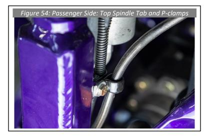
**77.** For the passenger side, attach the second p-clamp around the brake line and the second p-clamp around the wheel speed sensor to the middle spindle tab in a similar manner as the previous step (see Figure 55).
