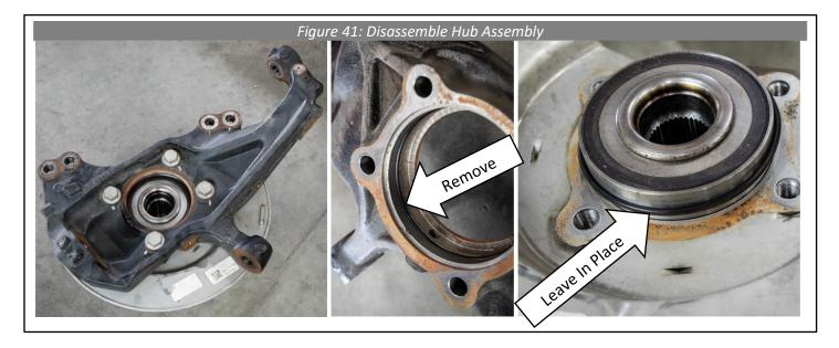
**55.** Transfer all the parts to the appropriate Cognito spindle, **8760** is the driver side and **8761** is the passenger side. Make sure that the bore and O-ring groove of the Cognito spindles is clean and free from debris. Torque the bearing hubs to the spindles with the factory bolts to factory torque spec 133 ft-lb (see Figure 42).
