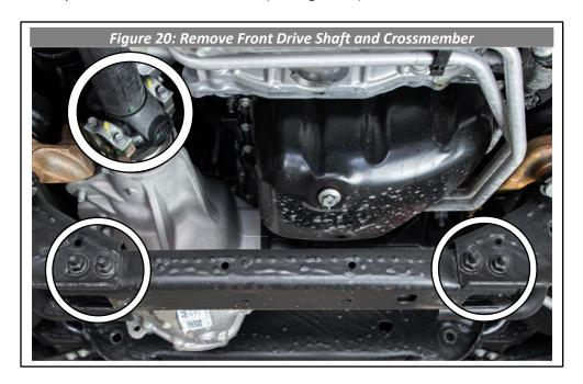
**25.** <u>Skip this step for 2WD vehicle.</u> Support the front differential with a transmission jack to prepare to lower it from the frame It is best to use a bracket on a transmission jack that will bolt or clamp to the front differential so it will stay fastened to the jack (See Figure 21). Lower cautiously.
