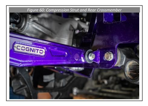
**84.** Loosely bolt the <u>2880</u> compression strut frame bracket to the other end of the driver compression strut using the 1/2" hardware located within the <u>HP9040</u> hardware pack.
