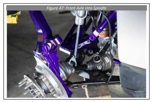
**66.** Place the <u>6688</u> Front Axle Spacers between the differential mount axle face and the front axle. Be sure that the center bore is place snuggly against the axle face on the differential mount axle face. Fasten the flange bolts using a rachet and 19-mm wrench and torque to factory torque spec 58 ft·lbs (see Figure 48).
