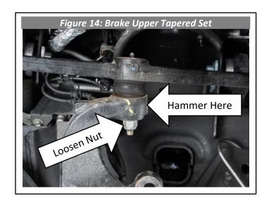
Install Sheet #7299 | Cognito 10-12" Front Suspension Lift Kit for 2020 GM 2WD/4WD 2500/3500
