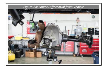
27. <u>Skip this step for 2WD vehicle.</u> After removing the differential from the vehicle, cut or grind a notch out of differential case. The notch will be made near the bolt hole closest to the yoke on the driver side of the differential. (See Figure 25)
