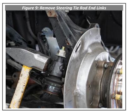
**12.** Use a 24mm socket to loosen the lower control arm ball joint but do not completely remove the nut. Now break the tapered set apart by using a pickle fork or hit the spindle casting with a hammer (See Figure 10).
