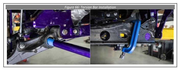
**96.** Adjust the torsion bars using the adjuster nut and bolt so that the front ride height is even on the passenger and driver side (see Figure 67). Do not over crank the torsion bars to try and gain too much height. **Never tighten the torsion key adjuster screws while the vehicle is on the ground.**
