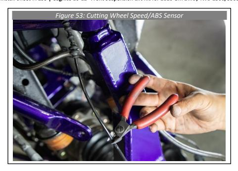
**74.** Locate the <u>110-70077</u> Front Wheel Speed Sensor Extender Kit. Splice the wheel speed sensor wires and use the butt connectors to crimp together the gray wire extensions included in this kit to the ABS wires. Do this process on both sides of the vehicle.
