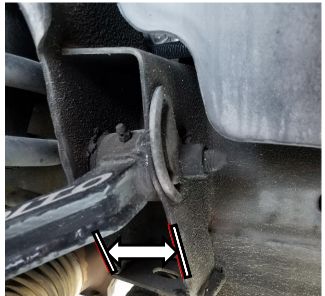
Figure 2: Factory Frame Service Perch Removal - After
