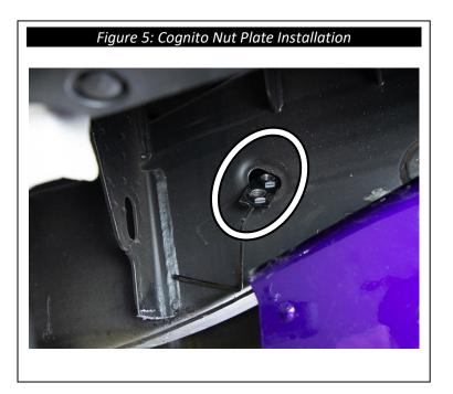
9. Locate HP9205 and find the two (2) 1/2" flat washers, two (2) 1/2" lock washers, and two (2) 1/2"-13 x 1.25" bolts. Install the lock washer between the flat washer and the bolt head and bolt the frame mount bracket to the nut plate, see Figure 6. Tighten and torque these two (2) bolts to 90 ft-lbs. Revision Date: 8/26/2021
