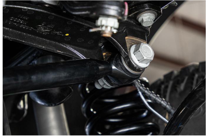
Figure 11: Installed Track Bar
