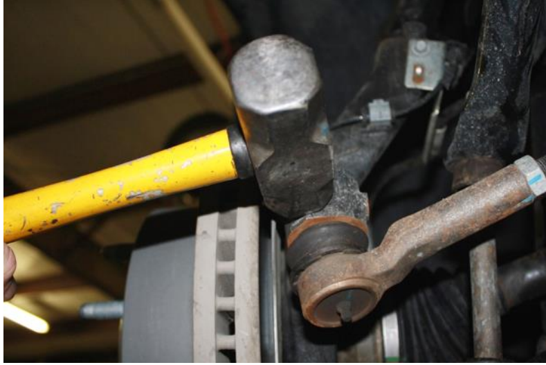
Figure 6: (OPTIONAL) Remove Tie Rod from Passenger Spindle
