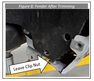
5. Trim the fender liner so that it will sit above the tube shown in figure 9 for GMC trucks, then install one of the bolts removed during step 3 into the hole shown to secure the fender liner. For Chevy trucks, cut the liner at the bottom of the tube and use a self tapping screw in the location shown in figure 9 to secure it.
