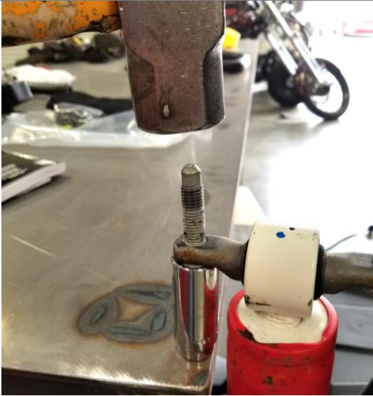
Figure 5: Remove OEM Shock Studs
