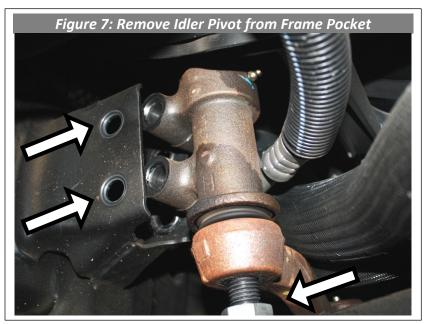
Note: There are two different center link designs used by GM, one with the rubber isolator bushing shown below, and one without. If your center link has a rubber bushing as shown, discard 6402 spacer included in the kit.
