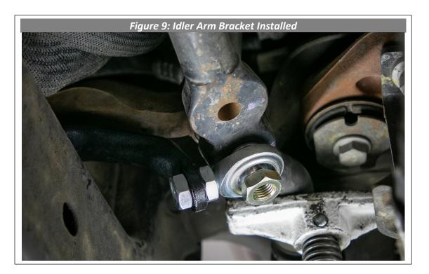
10. Reinstall the idler pivot into it's frame mounting pocket and reinstall the two bolts, tightening to 122 Ft.-lbs. Then tighten the idler pivot nut to 200 Ft.-lbs.
