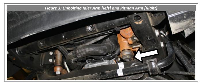
5. Support the steering box with a jack, then remove the 3 bolts holding the steering box to the frame using a 21mm socket. The steering box can then be jacked up to give more room to work above the crossmember. See figures 4 and 5.
