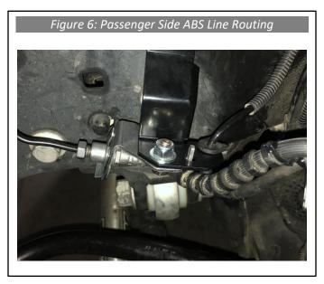
6. Once the brake lines are in place, turn the steering wheel all the way to passenger side of vehicle and check to make sure the brake lines are not interfering with springs, brackets, or tires. Repeat with the wheels turned all the way to the driver side of the vehicle.
