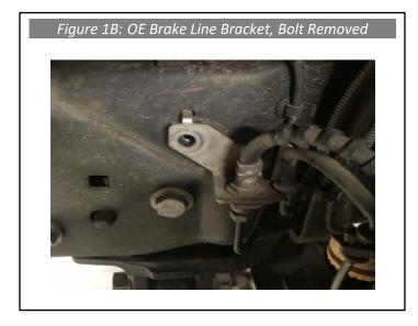
2. Remove the ABS line from both driver and passenger side OE brake line brackets by pulling the rubber boot out of the containment slot (Figure 2 A/B).
