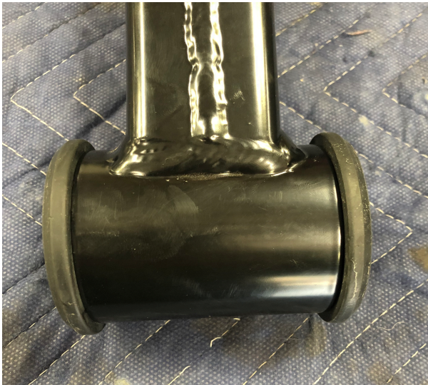
Figure 21: Traction Bar Bushings Installed
