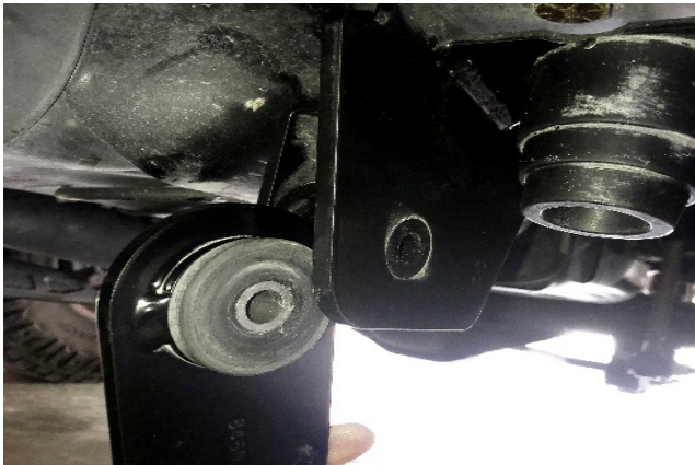
Figure 16: Assemble Shackles to Frame Mount
