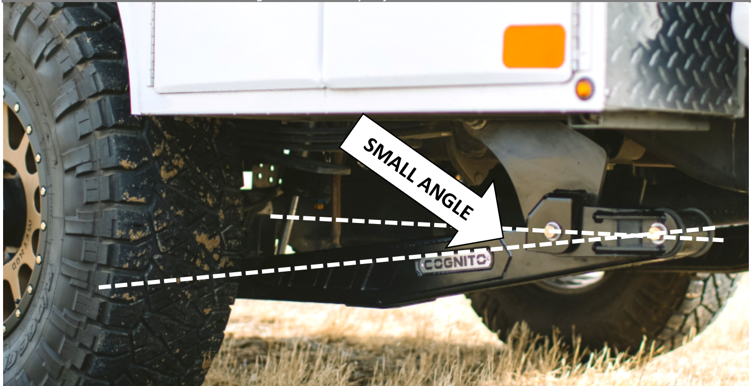
Figure 31: Correctly Adjusted Traction Bars
