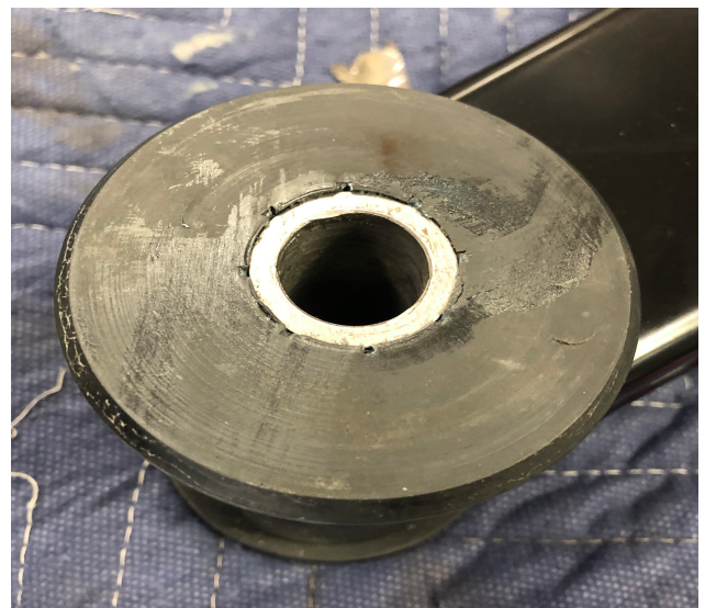
Figure 24: Crush Sleeve Installed
