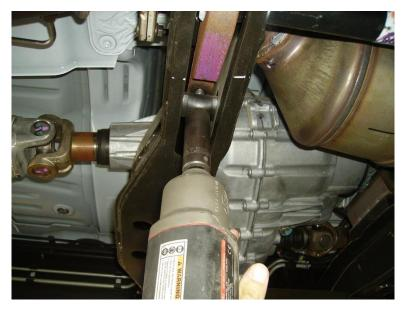
Figure 1: remove torsion bar adjusting bolt
