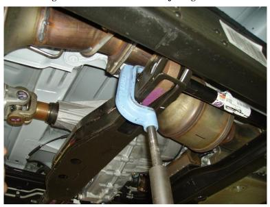
Figure 2: load torsion bar to remove adjuster nut
