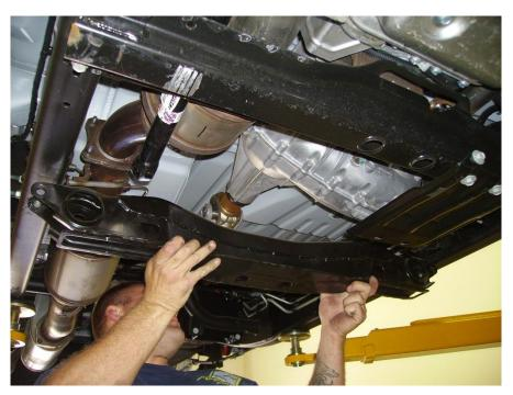
Figure 4: Remove factory torsion bar crossmember
