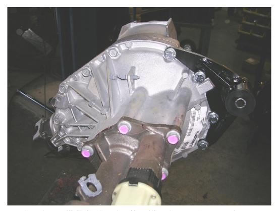
Figure 17: part #8151 Cognito Driver Side Differential Mounting Bracket installed
