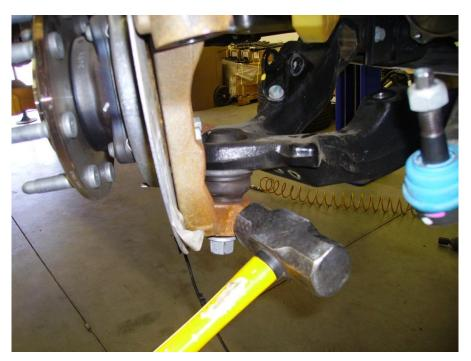
Figure 9: removing lower control arm.
