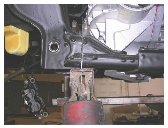
Figure 13: Cutting the frame pocket.
