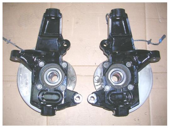
Figure 24: Spindle and bearing hub assembly.
