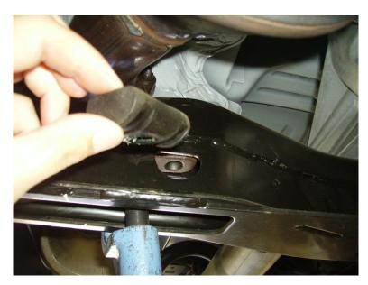
Figure 3: adjuster nut removed
