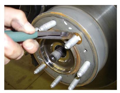
Figure 6: Remove clips from all 4 corners of vehicle. MUST DO for aftermarket wheels.
