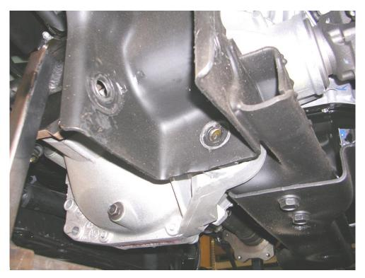
Figure 11: Lower bolt removed from front differential prior to making frame cut.
