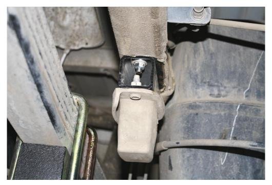
Figure 28: Rear bump stop spacer
