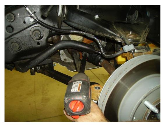
Figure 8: Remove CV axles on 4wd vehicles
