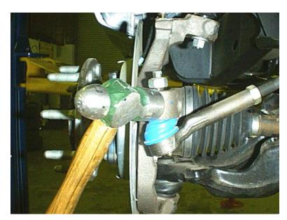
Figure 7. Remove tie rods from spindles.
