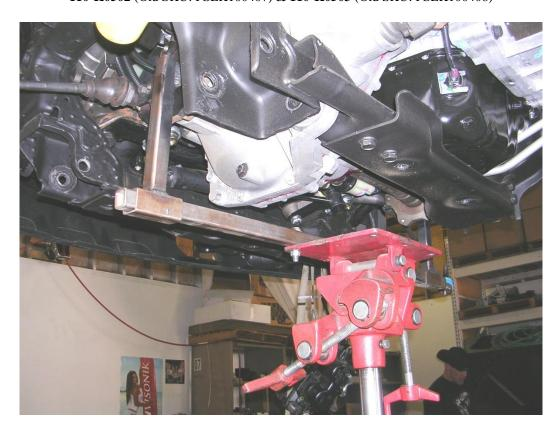
Figure 12: Supporting the front differential before cutting the frame.
