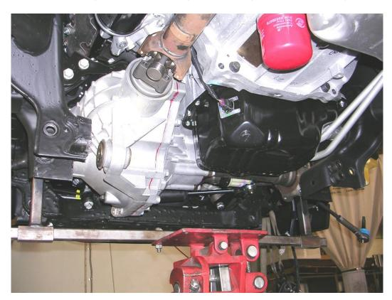
Figure 14: Factory crossmember and frame section removed.
