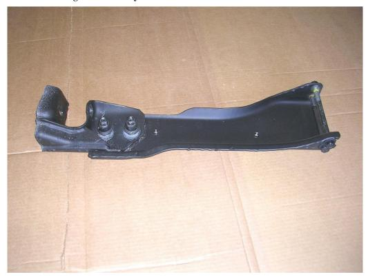
Figure 15: Factory crossmember and frame section removed.
