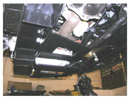
Figure 22: Cognito Skid Plate during installation
