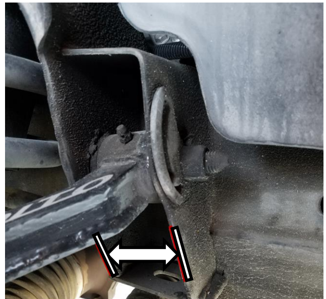
Figure 2: Factory Frame Service Perch Removal - After
