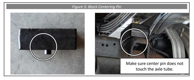
**10.** If the block is tapered, the tall end needs to be towards the <u>rear</u> of the vehicle. This will pitch the pinion angle up toward the transmission. If the block is straight, the hole on the top of the block may be offset from the centering pin on the bottom. If this is the case, orient the block so that the pin is offset <u>forward</u> of the pin in the leaf pack. The centering pin on the leaf pack should fit snugly into the hole in the top of the block (See Figure 6).
