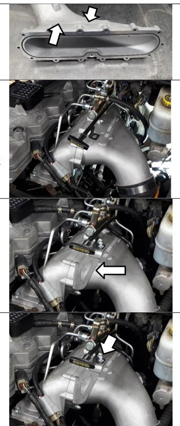
Be sure to plug in MAP sensor, and any other sensors installed on manifold at this time.
