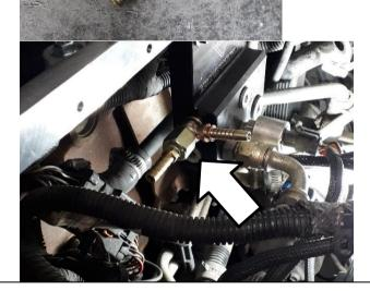
Re-install cp3 return pipe onto pump, and connect all the return banjo fittings with supplied 5/16" hose and clamps (1604031 & CTL-8.5).
