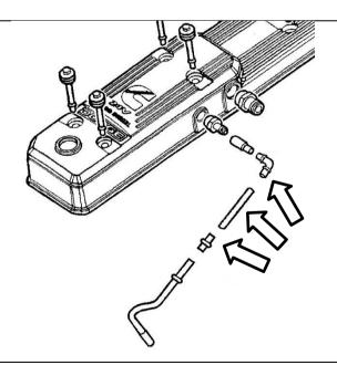
Route factory injector harness towards front of engine. (2005 model shown). 2003-05 model years (1500740
