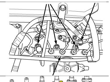
Remove CP3 return / fuel rail return hose assembly. Set aside, it will be reused in following steps.
