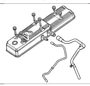
Install Upper Intake manifold (1405800), using M8x30 fasteners (1900015).
