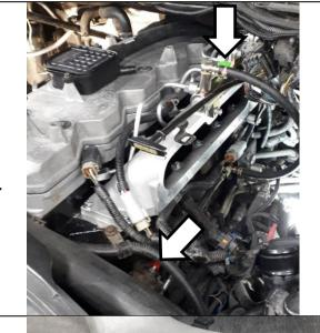
Install supplied O-ring (FT-0413965) into groove on lower intake manifold (1405801).
