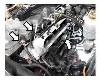
Insert fuel feed line (1405809) from CP3 pump to Fuel rail. Leave nuts loose for now, to aid in manifold install.
