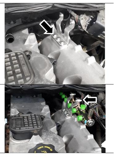
Install fuel lines starting at cylinder No. 6 and moving forward to cylinder No. 1. Install the following respective fuel lines:
