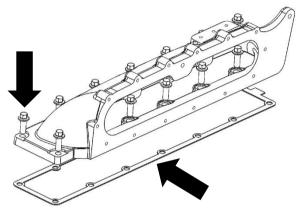
Install fuel rail bracket (1405802), using three [3] M6x16 fasteners (FT-0161811).
