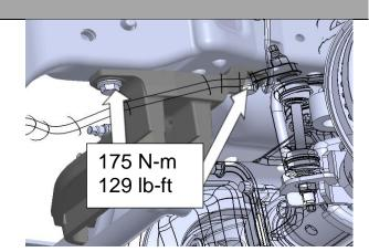
Install BD track bar bracket using the five OEM track bar bracket -to-frame nuts and bolts.
