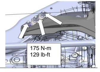
Install Track-bar into BD track bar bracket using OEM bolt and nut.
