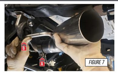
For the best tip fitment, align the barrel style tip clamp to cover *only* the slot, shown by **Arrow A**
