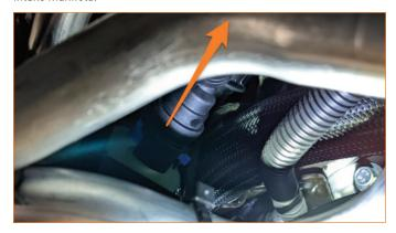
09. With both sides disconnected, the PCV line can be removed.
