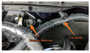
03. Unthread the plastic zip tie mount, this part will be reinstalled later.
