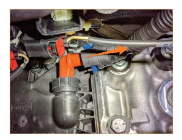
**08.** Remove PCV line quick-disconnect fitting the rear of the intake manifold.
