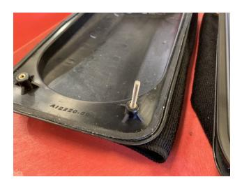
Once the cuts are done. Reattach the hood liner to the vehicle. Push in a Hood liner rivet (P) in each corner. This will make it easier to remove the liner in case adjustments need to be made.
