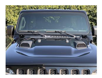
If extreme weather conditions arise such as heavy snow, dust or other debris grill plugs have been provided to prevent these elements from entering the hood scoops.
