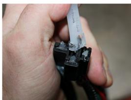
B. Place wire from ADD-A-CIRCUIT 46044 and WH-1006-3 into butt connector. Using crimping tool connect ADD-A-CIRCUIT 46044 and WH-1006-3 with butt connector. Install 46251 to ADD-A-CIRCUIT 46044 bottom slot (near wire that feeds additional circuit.
