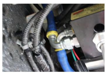
**H.** Remove the water-in-fuel sensor from the OEM fuel filter housing, install RVC-38 onto the WIF sensor. Reconnect WIF sensor plug to the wire harness on the truck, secure wiring with cable ties.
