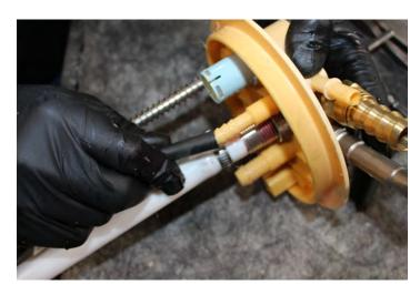
**Q**. Install FL-1009 onto the OEM engine feed barb, this will be the larger of the 2 plastic barbs. Reconnect the fuel level sending unit electrical connector and secure the tubing/wiring together with the supplied cable ties.
