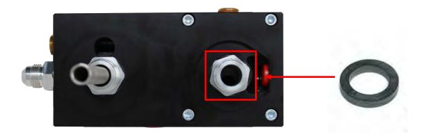
Note: O-Ring must be put back on suction side of pump. Failure to do so can result in priming issues, cavitation, or pressure loses.
