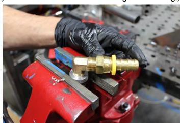
L. Install QD-1002 onto the OEM suction line on the fuel tank module.
