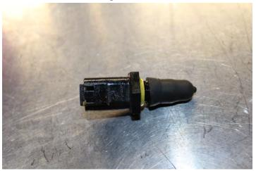
**I.** Using electrical tape, seal the OEM fuel pump connector to prevent road debris from entering. Reinstall the OEM fuel pump debris shield. Secure wiring from OEM connectors with cable ties.
