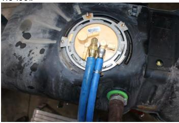
**S.** Remove and discard the OEM fuel feed line from the truck, this will no longer be used.
