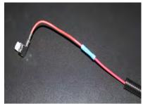
**C.** Secure relay and fuse in an upright position, as shown, to prevent moisture from entering. Be sure to use supplied dielectric grease on relay pigtail.
