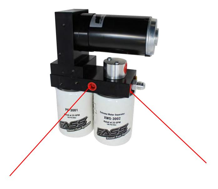
Note: The Red Plastic Plugs located in the "H" ports can stay in place fuel will not flow through these ports. Coolant can be plumbed into these ports to heat the fuel in the winter months.
