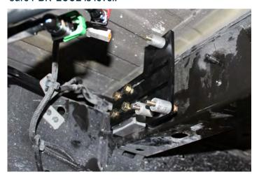
**E.** Install the FASS onto the (3) 1/4 mounting bolts and tighten accordingly.
