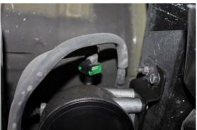
**D.** Remove the (4) bolts that secure the OEM fuel filter housing and remove the housing from the truck.
