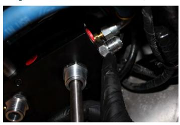
**E.** Install the remaining section of FL-1002 onto PL-2003 using oil. Install PL-2003 onto the FASS engine feed fitting 10-300, in some cases it may be necessary to remove the FASS return fitting. If removed, be careful to not damage the FASS pressure spring!
