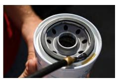
Extreme Water Separator - Install XWS-3002 on side of pump with draw tube in the middle of the filter nipple.
