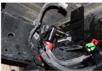
**D.** Install (3) 1/4" bolts with (3) WA-1001D spacers as pictured below. Tighten the (4) 3/8" bolts from step C, be sure PBR-2002 is level.
