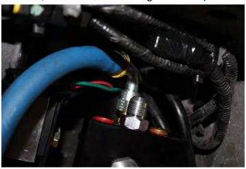
**F.** Install PLB-1212 into the OEM engine feed line, install FL-1002 from the FASS engine feed line onto PLB-1212 using oil. It may be necessary to trim FL-1002 to length!
