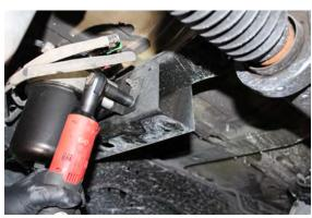
E. Remove the fuel tank skid plate, disconnect the fuel fill and vent tubes.
