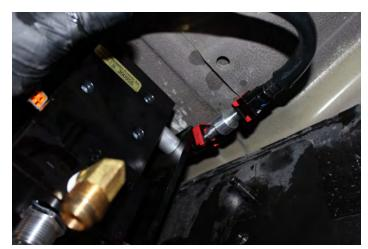
**C.** Install PL-1058 onto 10-302, route FL-1058 to PL-1058. Cut FL-1058 to length and install onto PL-1058 using oil.
