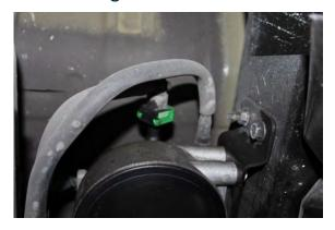
A. Remove the (3) 12mm bolts from the OEM fuel filter debris shield.
