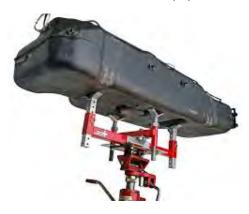
**G.** Remove and discard the fuel tank module shield, this will no longer be used. Clean the fuel module area then remove the lock ring on the top of the fuel tank. **This is spring loaded, so, holding it down while removing the ring will prevent the sending unit from popping up and possibly causing damage.**
