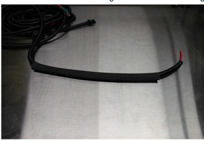
**E.** Route the single red wire of WH-1006-3 to the engine bay fuse panel on the passenger's side. Remove a fuse (maximum of 10A) that is "hot" when the key is on. Use a test probe to locate the "hot side" of the circuit in the fuse block. Install the Add-A-Circuit into the open location. Install the pulled fuse into the open space on the fuse tap.
