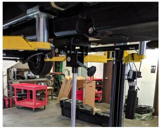
Remove the 4 bolts holding the 2 tank straps in place. Do NOT use a drill/air ratchet or you risk spinning the cage nuts.
