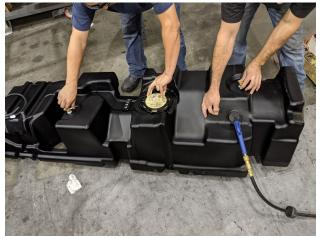
Install the fuel water separator onto the S&B Tank. To install simply push the separator onto the bracket that is installed on the S&B Tank. Don't worry about the Torx screw for now, it is easier to do that once the tank is in the truck.
