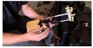
Place the black S&B o-ring in the o-ring groove and then carefully put the OEM sending unit(with OEM float attached) into the tank with the tab on the sending unit facing the arrow molded into the tank.
