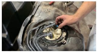
Remove the fuel lines from the hold down on the OEM tank. Simply pull upwards on the lines to pop them out.
