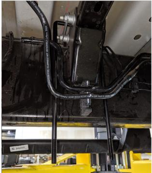
Slide the narrower U Bolt up and over the crossmember and position it against the driveshaft. Take your U Bolt positioning bracket and slide it on top of the cross member. Make sure the arrow is facing forwards. Align the holes on the bracket with the holes in the crossmember. Please proceed to step 24b and secure the bracket with the included nuts and bolts
