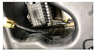
Reinstall the Torx water separator screw. If the screw will not easily thread in, your water separator isn't fully seated on the bracket. Wiggle it gently while looking through the bolt hole to see when it fully seats.
