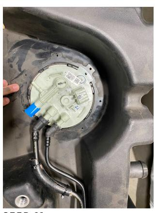
**STEP 11**Install the plugs over the vent rollover valve ports
