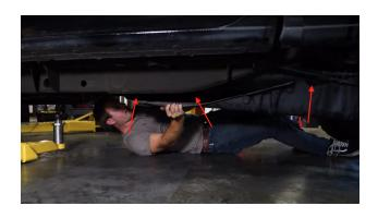
Disconnect and remove the return and feed fuel connectors.
