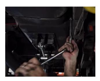
Lower the tank 3-4 inches and remove the 2 fuel lines that are going from the fuel tank sending unit to the fuel cooler.
