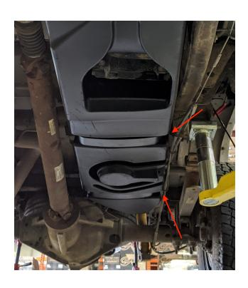
Install the S&B support bar in front of the S&B Tank. The hooks should be over the inside lip of the frame rail. Then by pressing up on the tank and pushing on the bar, slide the bar under the S&B Tank until it is in the groove on the S&B Tank.
