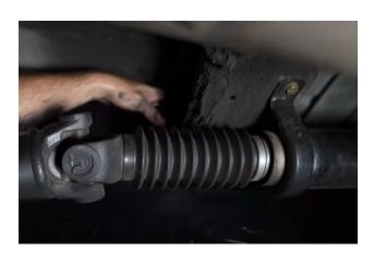
**STEP 13**Install the 2 S&B fuel tank straps.
