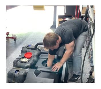
Remove the OEM sending unit from the OEM tank.
