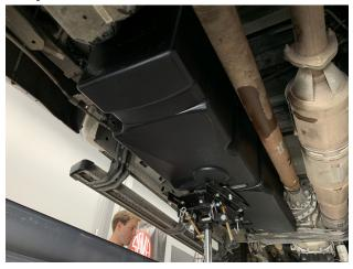
After you have installed the straps, install the front support bracket into the indentation on the tank. Place the washers over the threads and start the nylon lock nuts by hand. Tighten them evenly with a socket.
