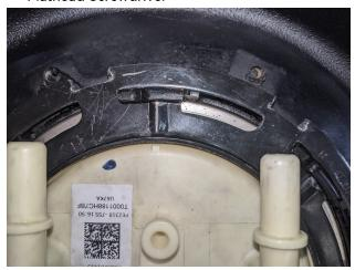
Transfer the OEM vent and fill hose to the S&B Tank and install them in the same orientation as they were installed on the OEM tank. If your S&B Tank is equipped with a long hose on the roll over vent, use the attached zip ties to attach the hose to the fill neck line. If not, don't worry about it.
