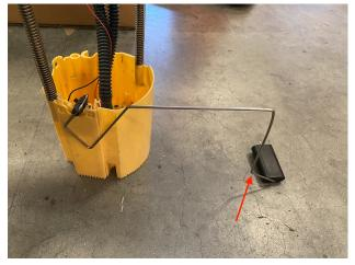
Replace the OEM fuel float with the included S&B Float. Place the S&B float into the fuel tank and hold the float off to the side so there's room for the sending unit bucket to pass through the hole. Once the float and bucket are inside the tank, connect the S&B Fuel float to the sending unit sensor
