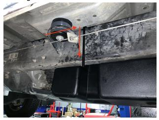
Center the S&B Tank on the jack and raise it until it is 6" from being in place. Reconnect the fuel sending unit electrical connector, blue return line fitting, and yellow feed line fitting. Make sure to push the locking tabs inwards on fuel line connectors.
