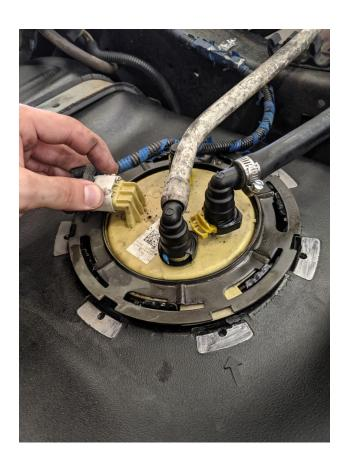
Reconnect the fuel line connectors by pushing down until they are fully seated. Push the fuel connector locking tabs back in once the connectors are fully seated.
