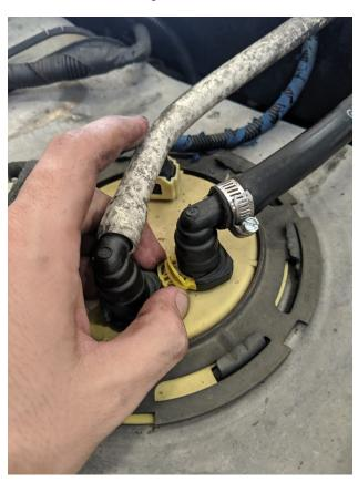
Now that the locking tabs are slide out, depress the upper tab, push down on the connector, then pull up. The connector should release. These connectors can sometimes be the hardest part of the install.
