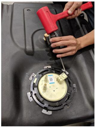
Make sure you rotate the locking ring until the rib on the OEM locking ring is fully seated into the indentation on the S&B receiving ring.
