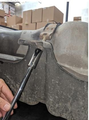
Remove the OEM tank from the skid plate. You may have to pry to get the OEM tank to pop out of the skid plate. Optional Tools
