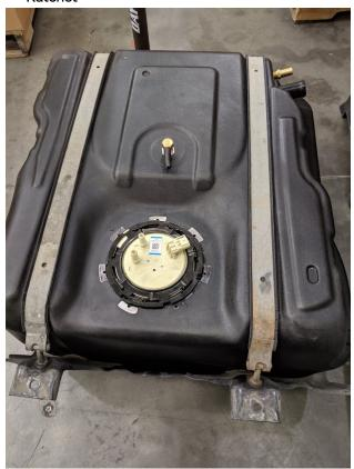
Position the S&B Tank on a jack and raise the tank until you are able to reconnect sending unit connections. Ensure the vent lines are positioned through the frame properly.
