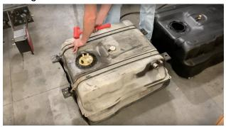
Place the S&B O ring into the groove on your S&B Tank.
