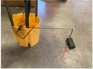
Applies to tanks with one rollover vent only. Insert the OEM sending unit with the S&B float attached into the S&B Tank. Align the tab on the sending unit with the arrow next to the opening on the tank.
