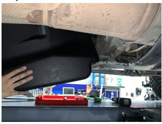
Using the OEM fuel tank strap bolts, start installing the straps(30 lb-ft). The S&B straps line up with the OEM straps and utilize the same cage nuts.
