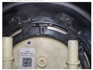
Transfer the OEM vent and fill hose to the S&B Tank and install them in the same orientation as they were installed on the OEM tank. If your S&B Tank is equipped with a long hose on the roll over vent, use the attached zip ties to attach the hose to the fill neck line. If not, don't worry about it.
